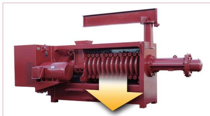
Depending upon Pressor capacity, the HCPR shaft can deliver up to 110 lbs. more fat per hour, with up to 25% lower residual fat in the crax.
